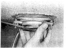
8 With the pressure removed, slide the retaining ring up and use a screw driver to pry off the snap ring to release the components
